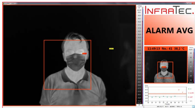
Should the previously defined temperature threshold be exceeded, an alarm is triggered via the software (here: simulated test alarm)
