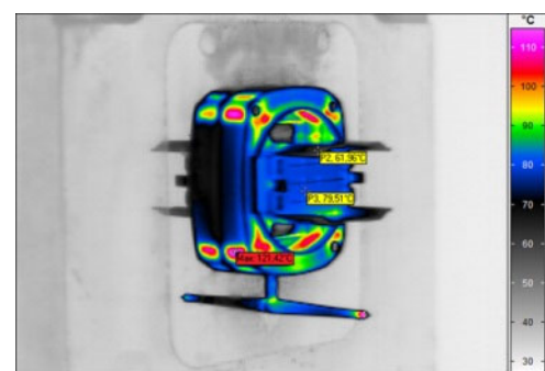
Fig 1 Thermogram of the moulded part at 60 °C mould temperature and 20 s totals cooling time
