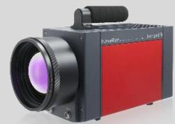
Non-destructive testing (NDT) – in contrast to destructive component testing – implies that the test application must not influence or reduce the usability of the test object in any way. Thermal imaging is a non-destructive, very efficient method. It enables the imaging detection of thermal radiation as well as the interpretation of the observed surface temperatures.
