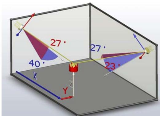
Fig. 8: Determination of the flame position by means of two PIA-903 detectors
