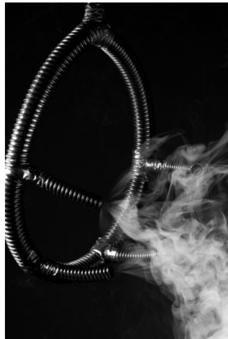
Figure 1. The circular suction device (prototype) displaying its efficacy to absorb plume in an experimental setting using a powerful nebulizer with excessive smoke production at low velocity.
